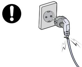
If a power plug is broken or a plug is cut or worn, do not use it.
