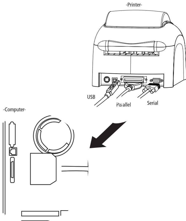
After making sure the printer is turned off, connect the printer to the PC.
