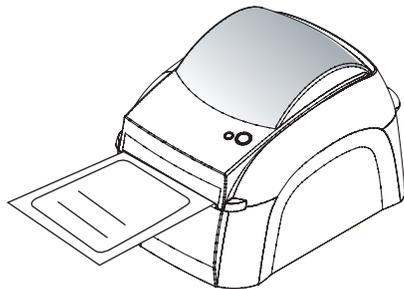
Printer sensor detects the size of the label, issuing the blank label.
