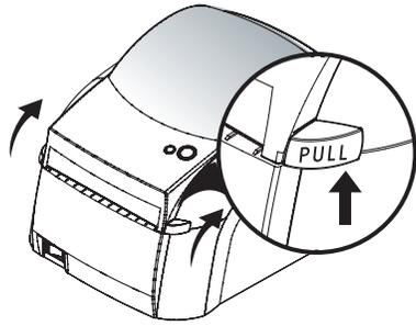
Open the upper cover by pushing the knob in the direction of the arrow.
