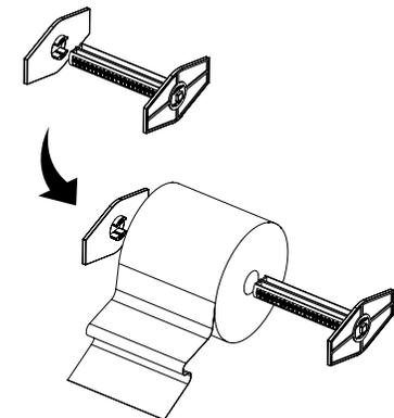
Insert the roll paper to the paper spindle as shown in the picture.
