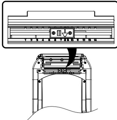
Locate notch sensor on the same number point- as the black mark sensor is indicating on.
