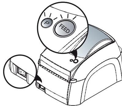
While you are pressing and holding 'P, FEED' button, turn on the power of printer.
