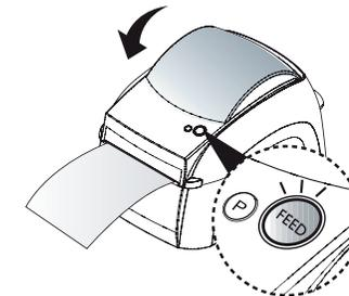
After the treatment has been done as picture above, the printer function normally once you press FEED button.
