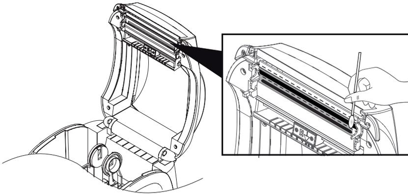
1. Use an applicator swab moistened with an alcohol solution to clean the print head and remove any dusts.
