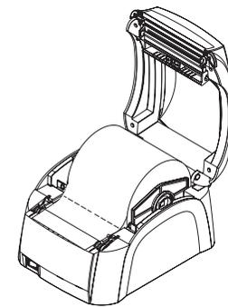
**\*\*Installation of the new paper when the printer is short of it\*\***
