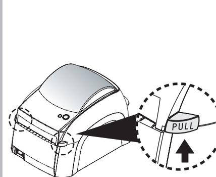
Turn off the printer and open the upper cover by pushing the knob in the direction of the arrow
