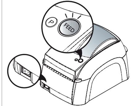
Press and hold the feed button while turning on the printer with power switch
