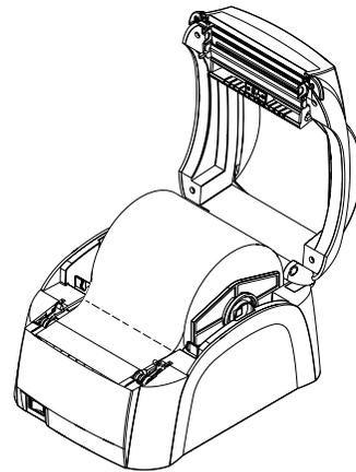
Adjust the paper width guide to meet the paper width
