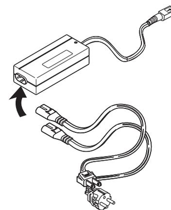
Connect the AC power cord to the power supply
