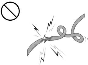
Do not bend the wire and do not allow the wire to be pressed by heavy object.
