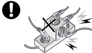
Do not overload the power plug into one outlet.
